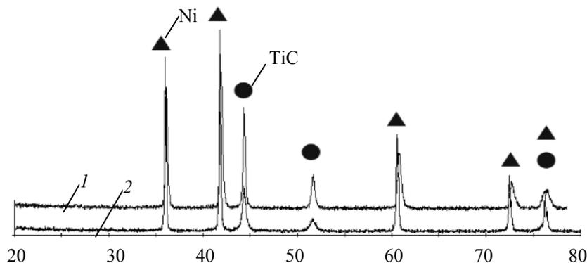
**Fig. 3. Results of X-ray phase analysis of the combustion products of a Ti+C+25% Ni mixture from the PTM grade titanium granulate:**
