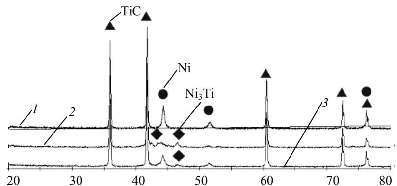
Fig. 7. Results of X-ray phase analysis of the combustion products of Ti + C + 25 % Ni granulated mixtures without gas flow from PTM titanium (1), PTM-1 titanium (2) and PTM and PTM-1 titanium in equal parts (3)
