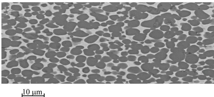
**Fig. 4. Microstructure of the Ti + C + 25 % Ni granules after synthesis**
