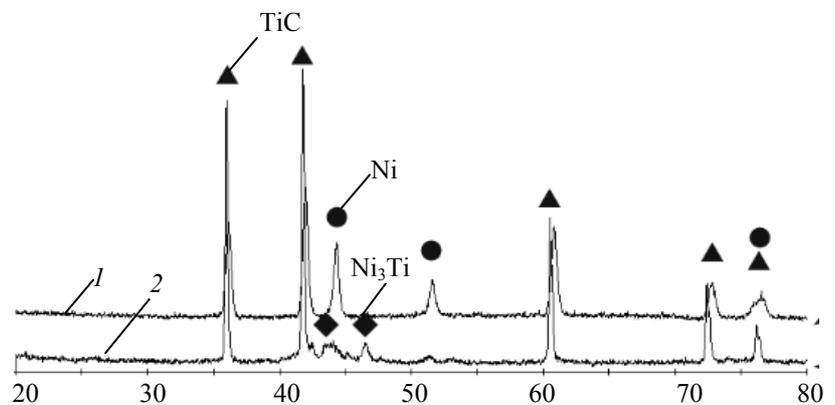
Fig. 8. Results of the X-ray phase analysis of the combustion products of the Ti + C + 25 % Ni granulated mixture from PTM-1/PTM titanium in equal parts without a gas flow (1) and in a nitrogen flow (2)
