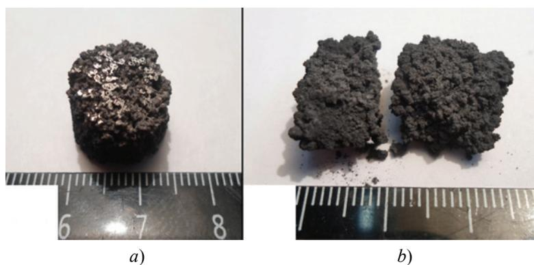
Fig 5. A cross section of the synthesis product of Ti + C + 25 % Ni granules in a gas flow: *a* – argon flow, *b* – nitrogen flow
