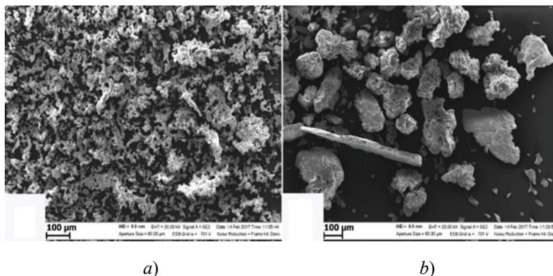
Fig. 6. Microphotographs of titanium powders of PTM (*a*) and PTM-1 grades (*b*)
