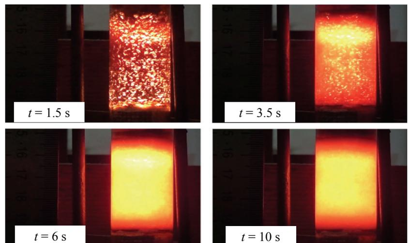
**Fig. 2. Shots of the process of synthesis of granulated mixture of nickel-bound titanium carbide with PTM titanium at different times (this time is measured from the moment of ignition)**
