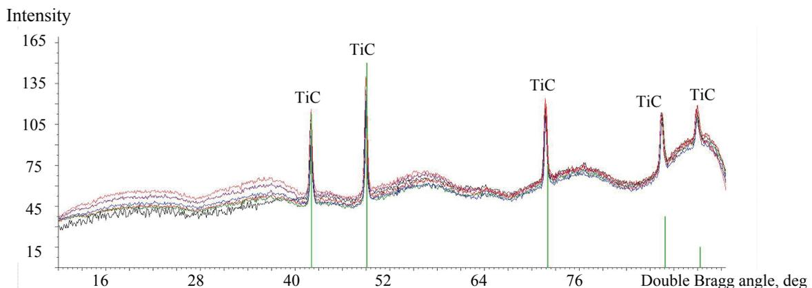
**Fig. 2. Results of X-ray phase analysis of powders produced by the SHS and SHS-grinding methods at rotor speeds of 120 and 240 rpm**
