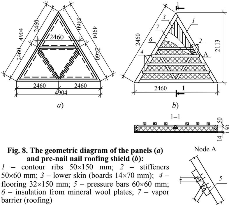
**Fig. 8. The geometric diagram of the panels (a) and pre-nail nail roofing shield (b):**
