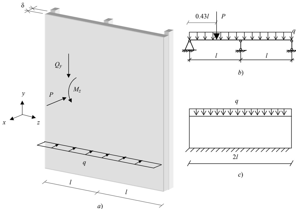
Fig. 10. The design scheme of the sheathing of the partition: a – general view of the partition design; b – in the horizontal plane; c – in a vertical plane
