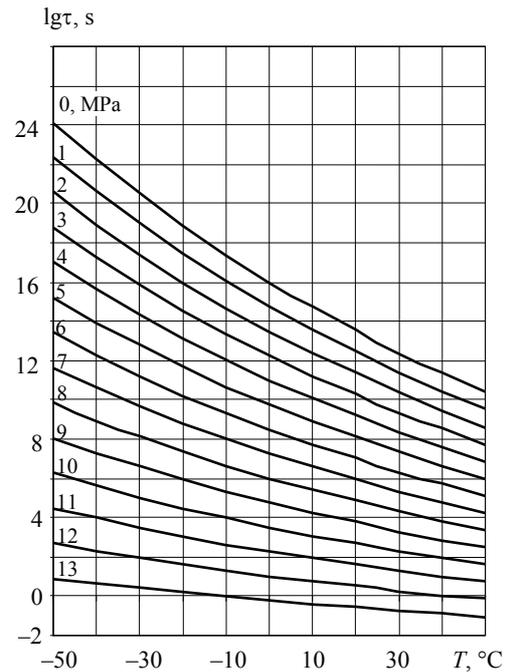
**Fig. 3. An example of a diagram for determining the transverse bending performance of chipboard with a density of  $650 \text{ kg/m}^3$**
