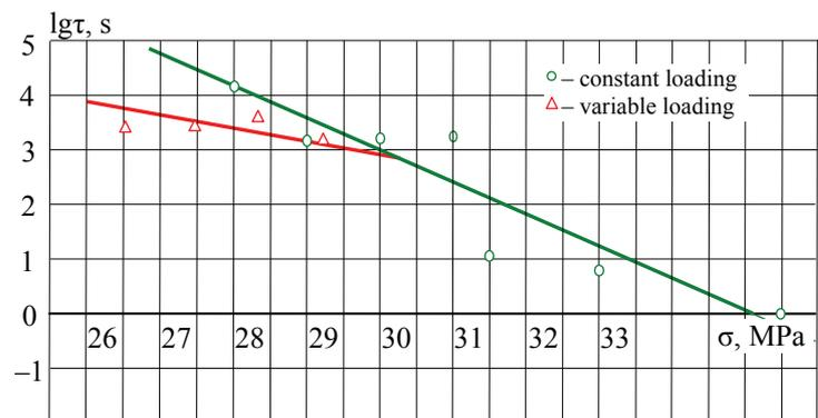
Fig. 6. The dependence of laminate durability on constant and variable stresses (with transverse bending) at a temperature of 20 °C
