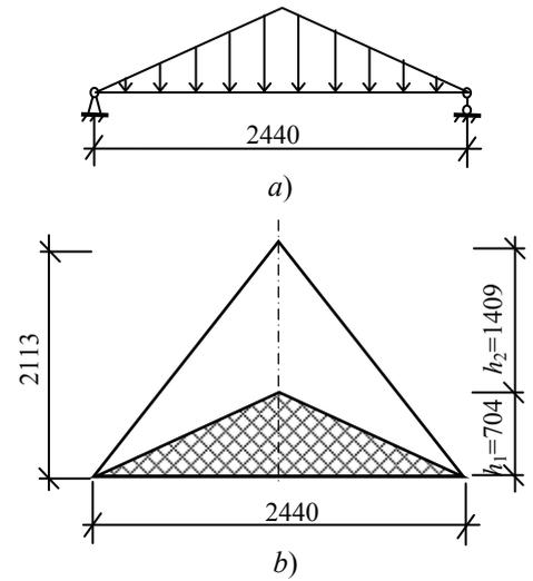
**Fig. 9. Estimated rib design (a) and estimated area (b)**
