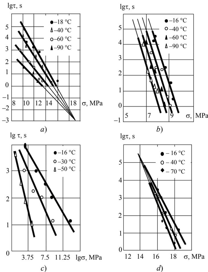
**Fig. 2. The durability dependence on stress during transverse bending for wood boards with a density:**
