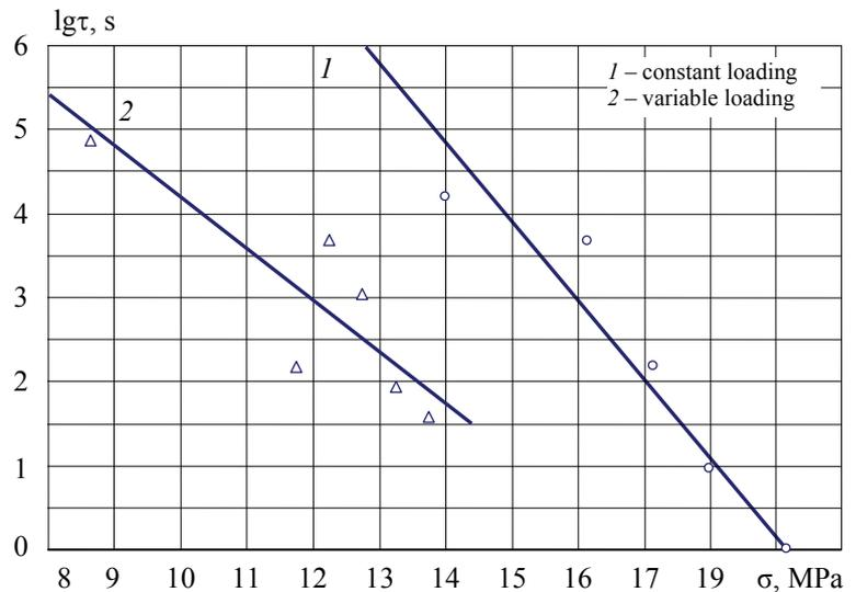
Fig. 5. The dependence of the chipboard durability from constant and variable stresses (with a transverse bend and a temperature of 18 °C)
