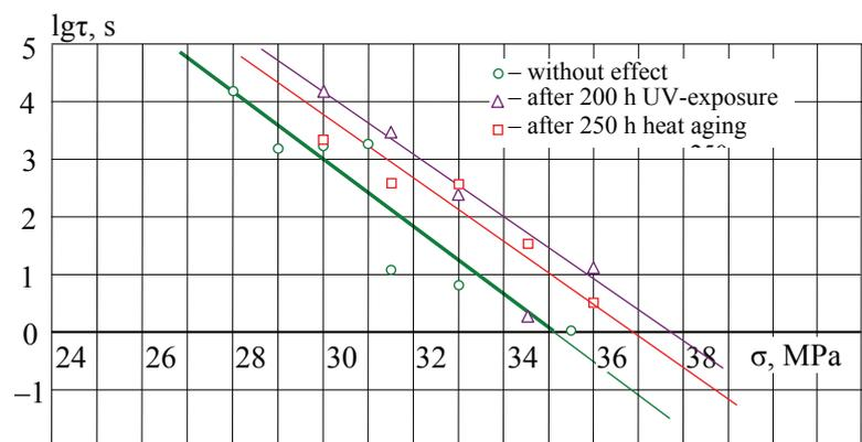
Fig. 7. The durability dependence on bending stresses for laminate Kronospan 31' after heat and photo aging
