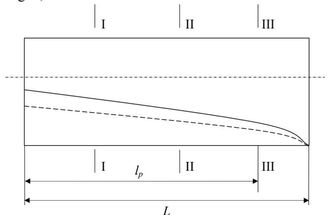
Fig. 2. The distribution of bulk material in the longitudinal section of the drum mixer of continuous operation
