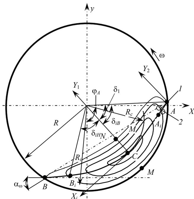
Fig. 1. Scheme for determining the character of movement of bulk material in the cross-section of the drum
