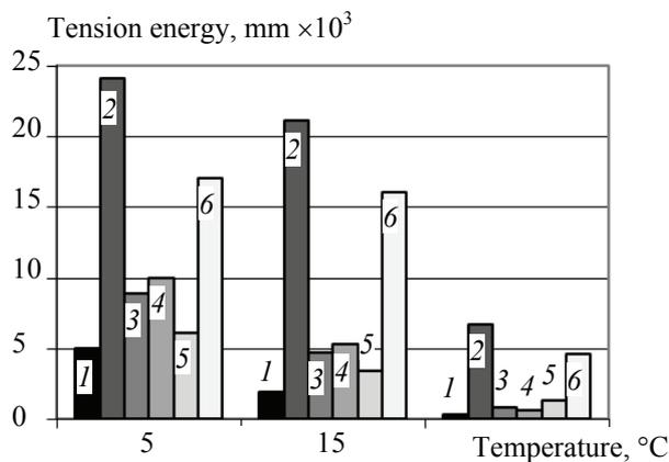
Fig. 7. The mean value of tension energy of Polish binders at temperatures of 5, 15 and 25 °C:
