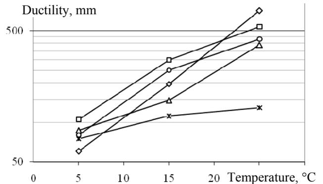
Fig. 4. Changes in ductility of Polish binders depending on the temperature:
