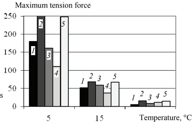
Fig. 6. The mean values of the maximum tension force of Polish binders:
