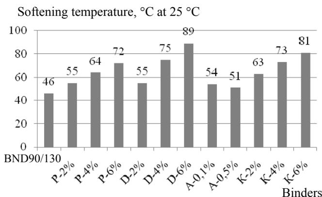
Fig. 3. Softening temperature of Russian bitumen binders
