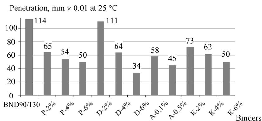
Fig. 1. Penetration of Russian bitumen binders at 25 °C
