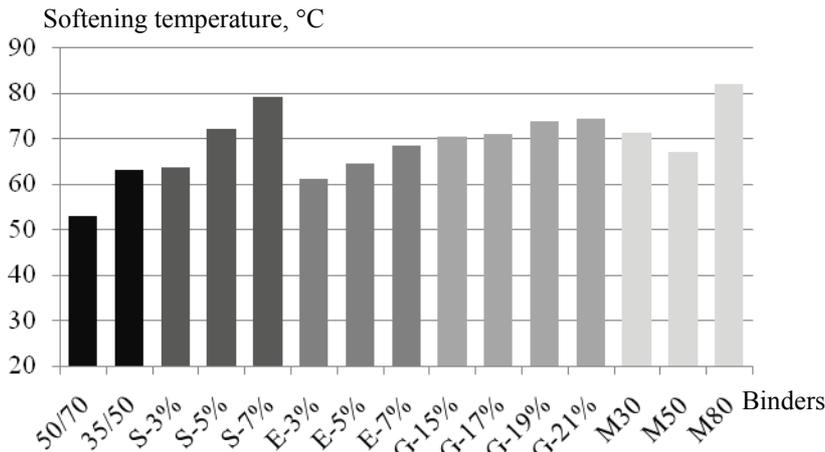
Fig. 2. Softening temperature of Polish bitumen binders
