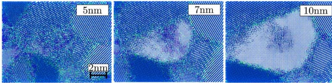
**Fig. 1. Molecular dynamics simulation of irradiation of nanodiamond particles by heavy fast ions with an effective stopping energy of 17 keV/nm depending on the particle size [5]**
