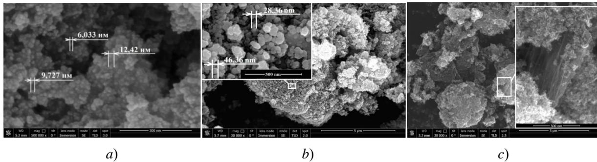
**Fig. 3. Microstructure of nanodiamond powder:**
