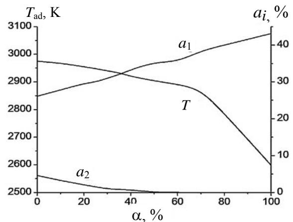
Fig. 4. Effect of  $\alpha$  on the calculated adiabatic temperature  $T_{ad}$ , mass fractions of metallic  $a_1$  and gaseous  $a_2$  chemical conversion products
