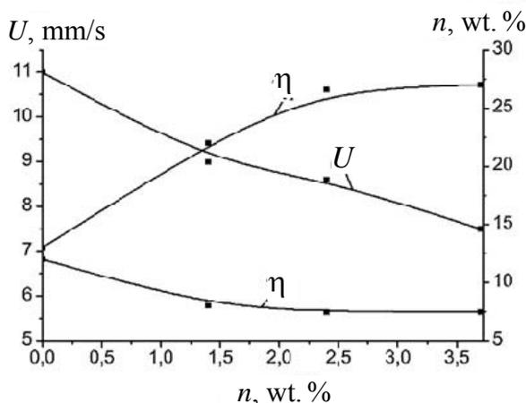
Fig. 2. Burning velocity  $U$ , yield of metallic phase  $\eta_1$ , and spread of combustion products (dispersion)  $\eta_2$  as a function of  $n$  ( $U = l/t$ , where  $l$  is the height of the mixture,  $t$  is the time of burning;  $\eta_1 = m/M_1$ ,  $\eta_2 = [(M_1 - M_2)/M_1] \times 100\%$ ,  $M_1$  is the mass of the initial mixture,  $M_2$  is the mass of the final combustion products and  $m$  is the mass of the metal ingot)
