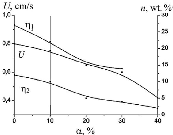
**Fig. 5. Burning velocity  $U$ , yield of metallic phase  $\eta_1$ , and spread of combustion products (dispersion)  $\eta_2$  as a function of  $n$**
