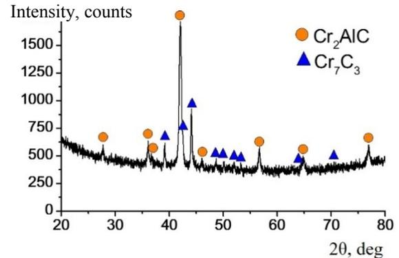
Fig. 3. X-ray diffraction pattern of the product obtained at  $n = 2.4\%$
