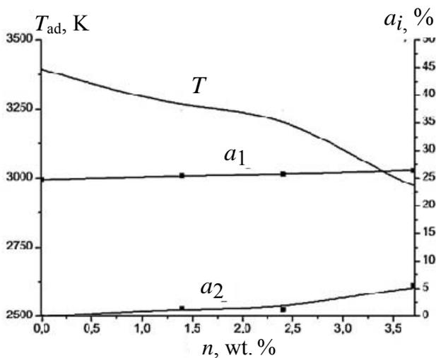
Fig. 1. Influence of the carbon content in the initial mixture on the calculated adiabatic temperature  $T_{ad}$  and mass fractions of metallic  $a_1$  and gaseous  $a_2$  chemical conversion products
