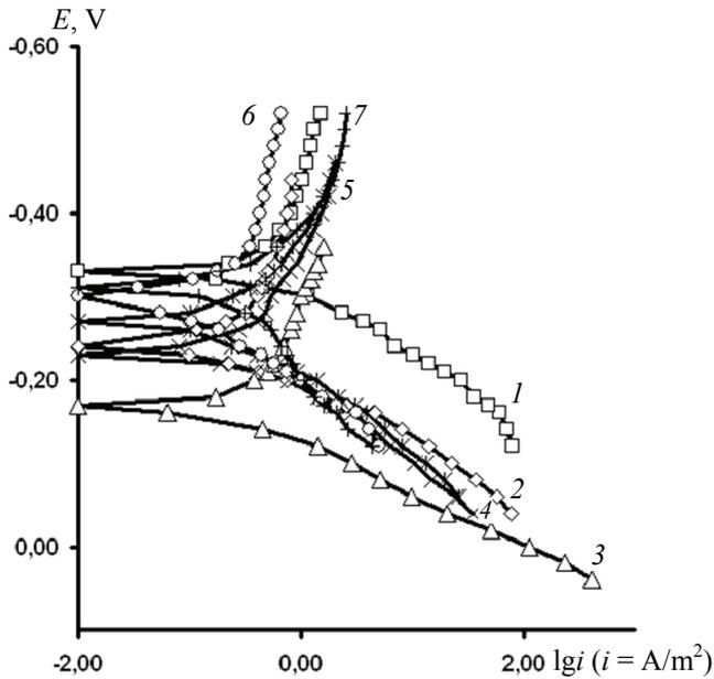
**Fig. 1. The carbon steel polarization curves in 0,5 M NaCl solution without (1) and under colza oil coating (2) and its compositions, wt.% SFAB: 3 – 2,5; 4 – 5; 5 – 10; 6 – 15; 7 – 20**
