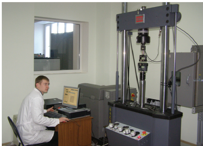
Photo 2. The study of nanostructured matrix tensile strength in the laboratory of micro- and macromechanical testing
