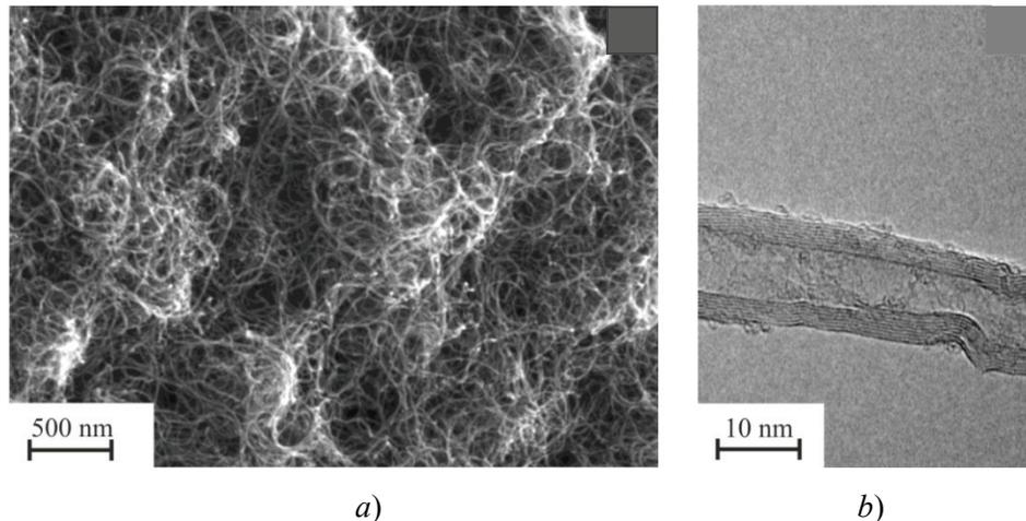
Fig. 1. SEM (a) and TEM (b) images of the “Taunit-M” MWCNTs
