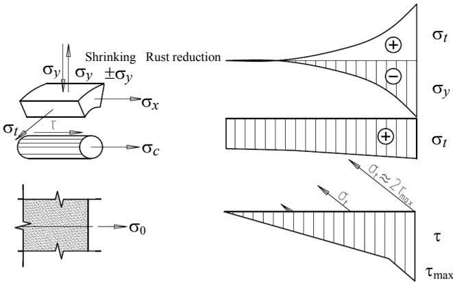
**Fig. 2. Stress-strain state between reinforcing rod and concrete in pull-out-test**
