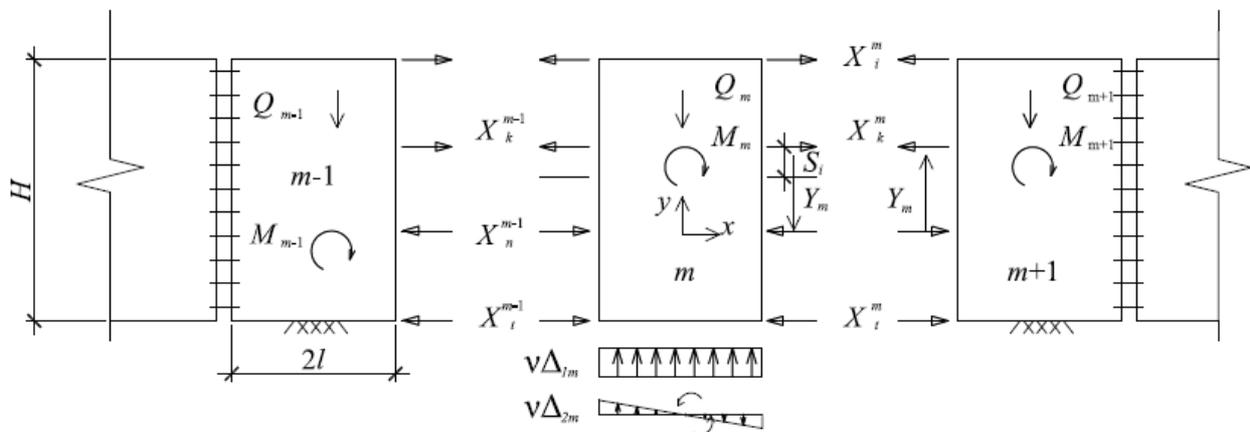
Fig. 1. Diagram of forces acting on a separate block of butt joint
