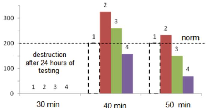
Fig. 4. The dependence of the swelling degree of the WEC samples on the duration of vulcanization with different content of water-swelling additive after 672 hours of testing: 1 – 80 PA; 2 – 70 PA; 3 – 60 PA; 4 – 50 PA
