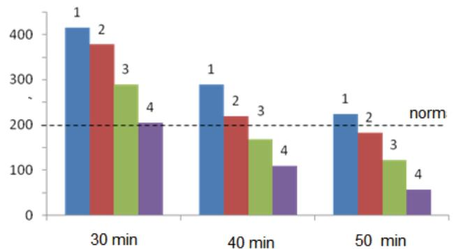
**Fig. 3. Dependence of swelling degree of WEC samples on duration of vulcanization with different content of water-swelling additive after 168 hours of testing:**
