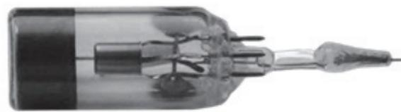
**Fig. 4. Cathodoluminescent lamp of a triode structure with an auto ionic cathode**
