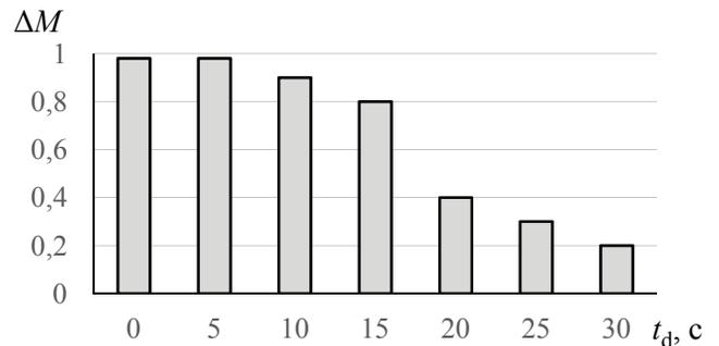
Fig. 6. The dependence of the crushed mass of products on the delay time before the application of mechanical treatment
