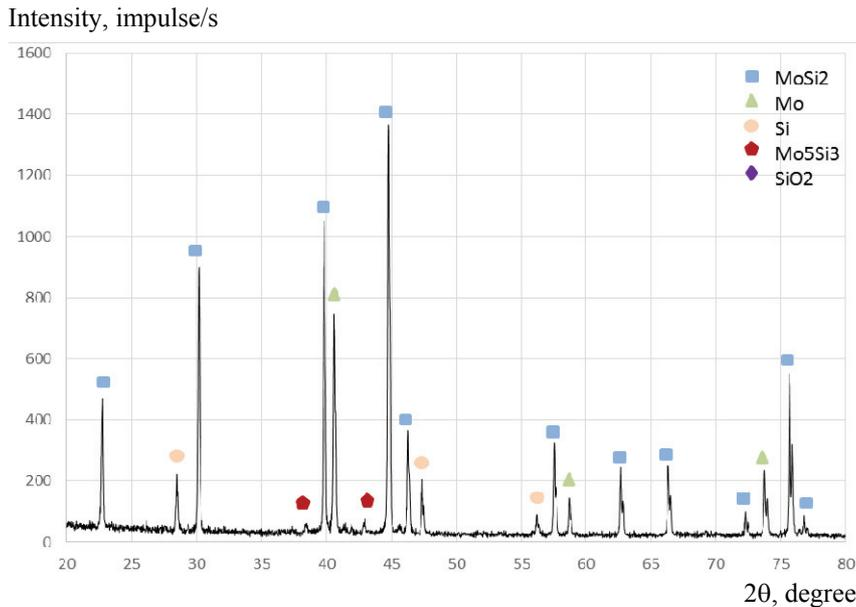
Fig. 4. Radiography of MoSi<sub>2</sub> after the mechanical treatment at  $t_d = 0$  s
