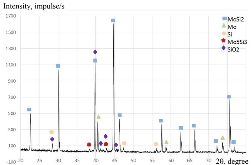
Fig. 2. Radiography of  $\text{MoSi}_2$  without mechanical treatment
