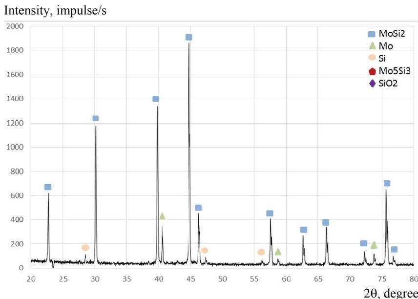
Fig. 5. Radiography of MoSi<sub>2</sub> after the mechanical treatment at  $t_d = 5$  s
