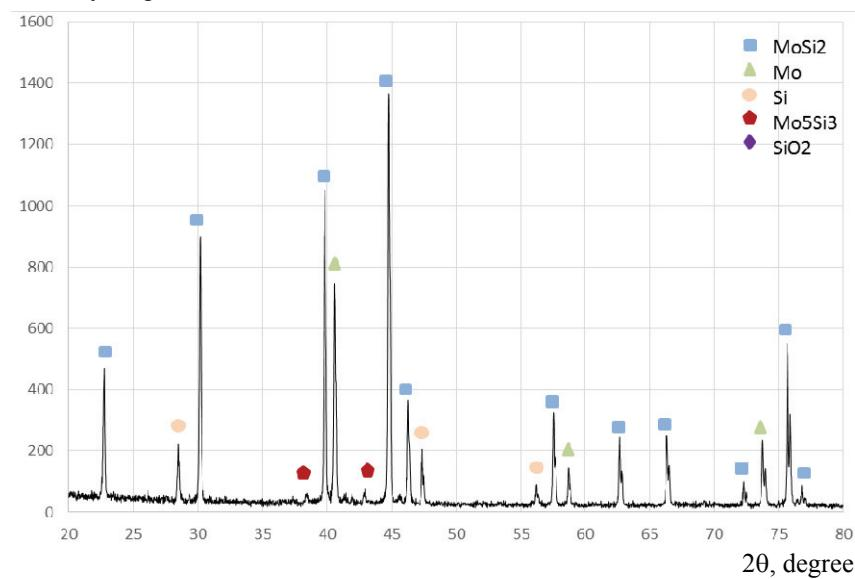
Рис. 4. Radiography of MoSi<sub>2</sub> after the mechanical treatment at  $t_d = 0$  s
