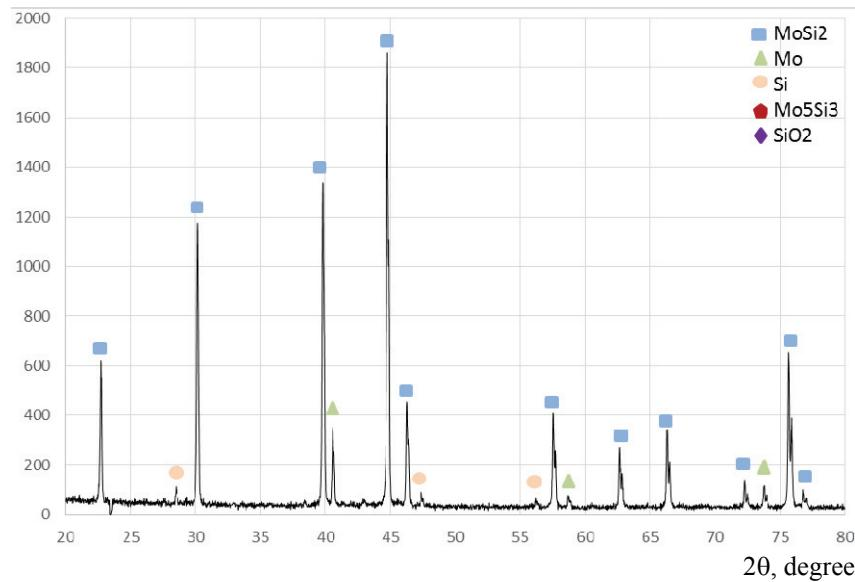
Fig. 5. Radiography of MoSi<sub>2</sub> after the mechanical treatment at  $t_d = 5$  s
