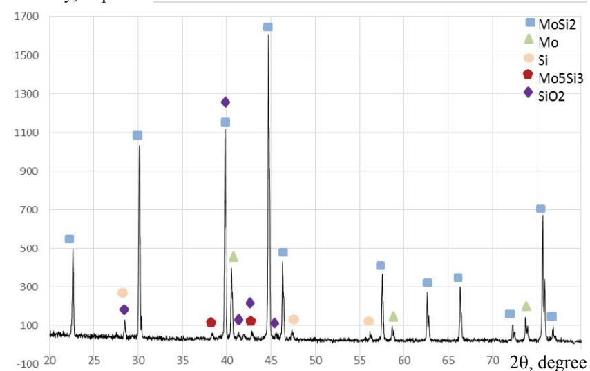
Fig. 2. Radiography of MoSi<sub>2</sub> without mechanical treatment**Experiment and discussion**
