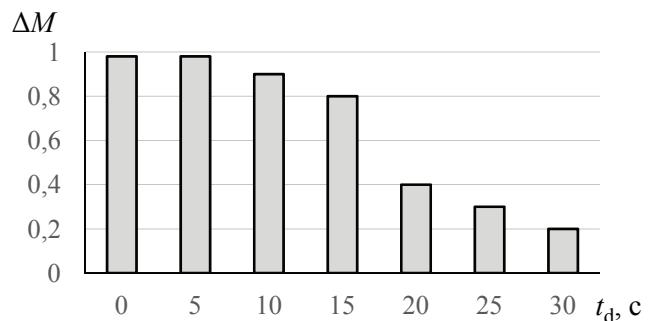
Fig. 6. The dependence of the crushed mass of products on the delay time before the application of mechanical treatment
